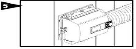
Attach solenoid valve to side of humidifier cabinet with flow arrow pointing up, using thumb nuts provided. Do not reverse brass fittings as valve will not function if flow is reversed. Assemble distributor tube so that it is directed into the center opening of the distributor trough cover. Connect 1/4" water supply tube to brass filter at inlet of solenoid. DO NOT USE PLASTIC TUBING IN CONTACT WITH ANY HOT PLENUM SURFACE OR DUCT. IF USING PLASTIC TUBING, USE TUBE SUPPORT PROVIDED.
