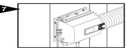
Connect drain hose to 5/8" spout on humidifier cabinet using hose clamp provided. Flun 5/8" hose to suitable drain such as floor drain, sewer or laundry sink. Be sure hose has continuous slope and is not kinked at any point.
