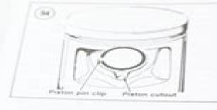
CHURCOSON If it is recoverary to sap the piston pin one the connecting rad, do no gentle with a block of wood or a soft-faced hammer. Afaile sure you support the perton to prevent the lateral shock from being transmitted to the connecting rod Described.
