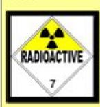
HRCQ is a high activity shipment transported in a Type B package. The package will always have a Yellow-Ill label regardless of radiation level. HRCQ shipments by highway will require the standard placard on a white square background with a black border as shown at left.
