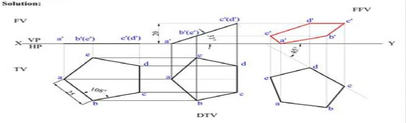
**Problem 28:** A pentagonal lamina having edges 25mm is placed on one of its corner on HP such that the perpendicular bisector of the edge passing through the corner on which the lamina rests is inclined at 30° to HP and 45° to VP. Draw the top and front views of the lamina.
